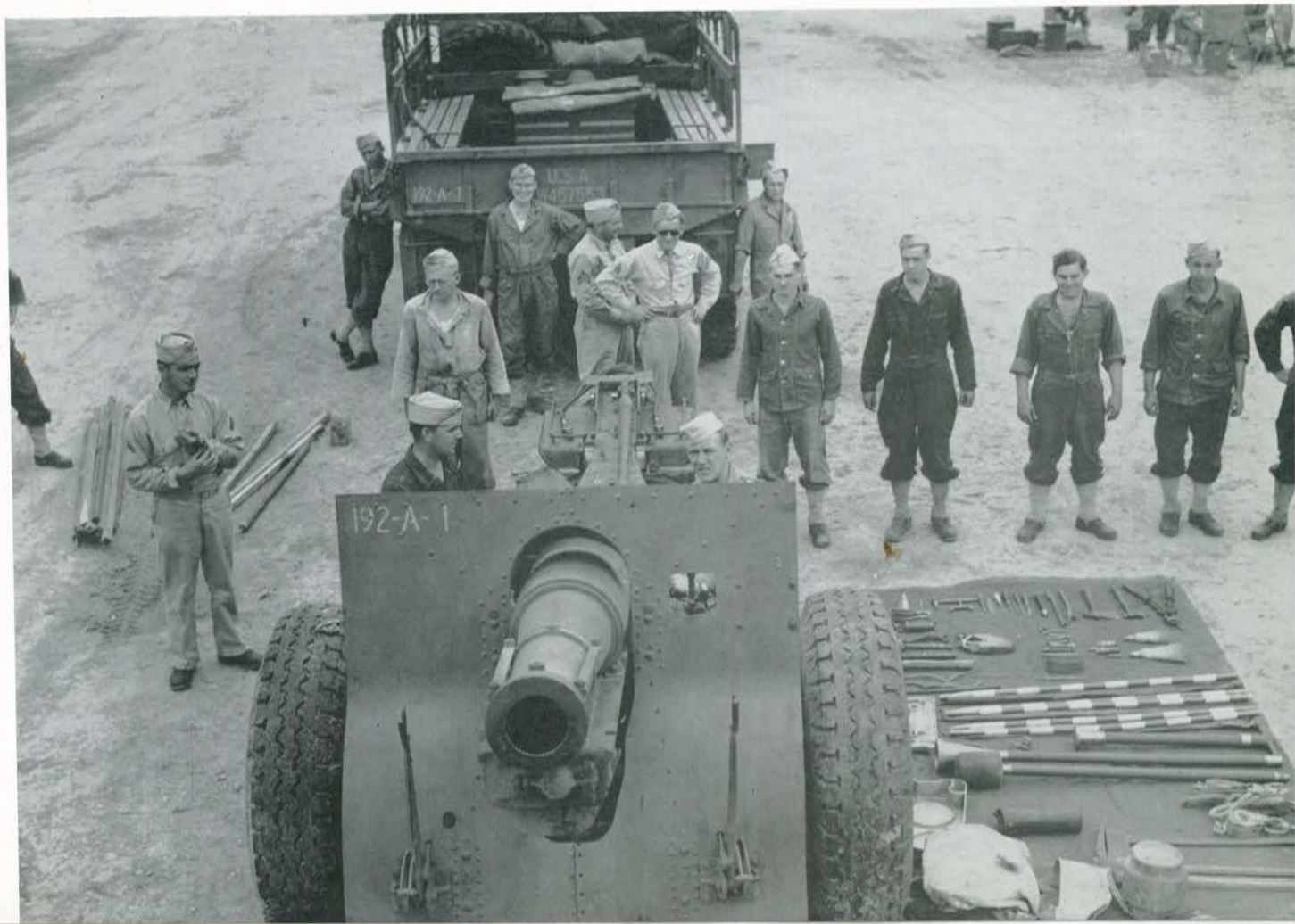
A 155-MM. HOWITZER AND CREW WITH ALL THE GADGETS NECESSARY TO ITS OPERATION
