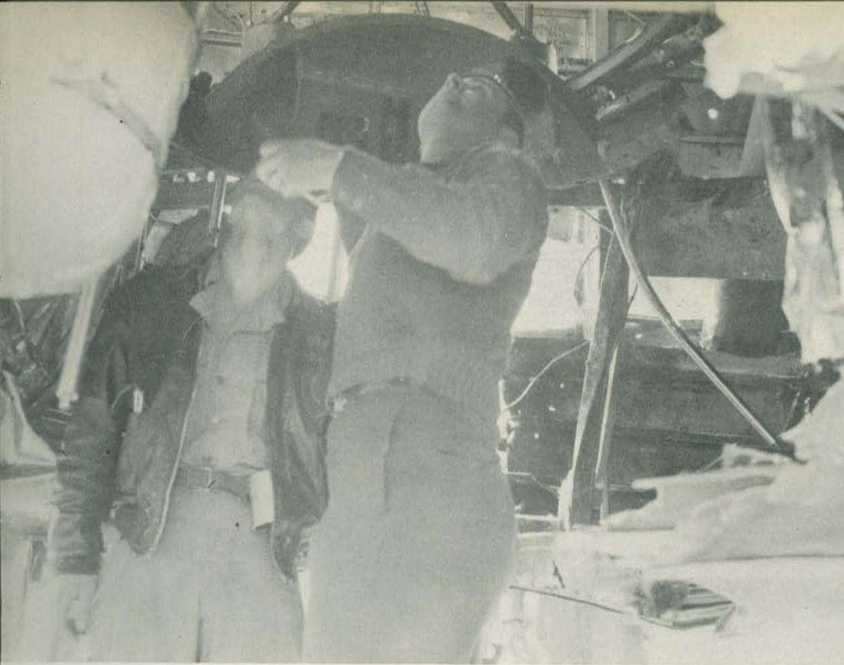
FLAK DAMAGE—A DIRECT HIT ON THE BALL TURRET.
