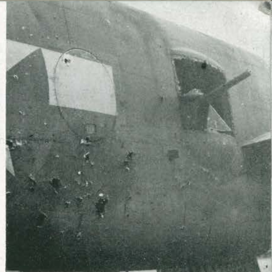
The other side of the same plane, where shell fragments ripped through the fuselage and splintered the window.
