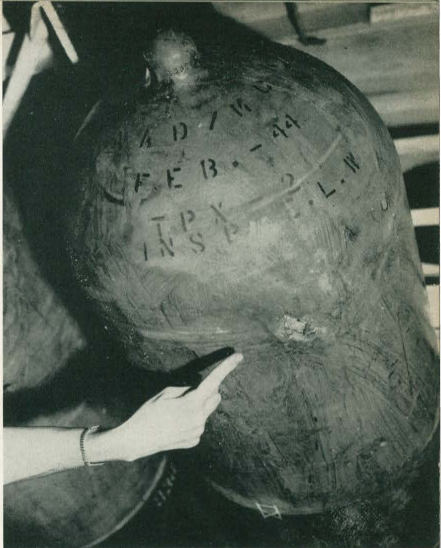
Shrapnel damage to warhead.
