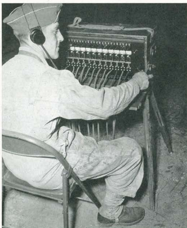
Testing lines by means of outdoor switchboard.
