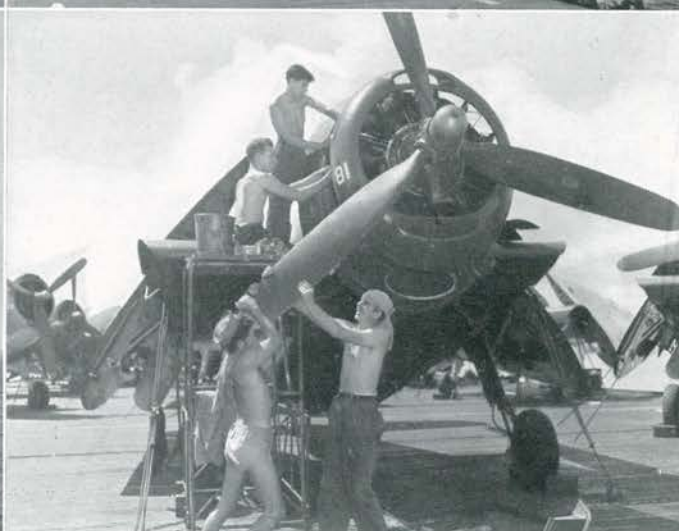
Top: Avenger takes a wave-off; below: Aviation mechs pull routine valve check on Avenger on flight deck.
