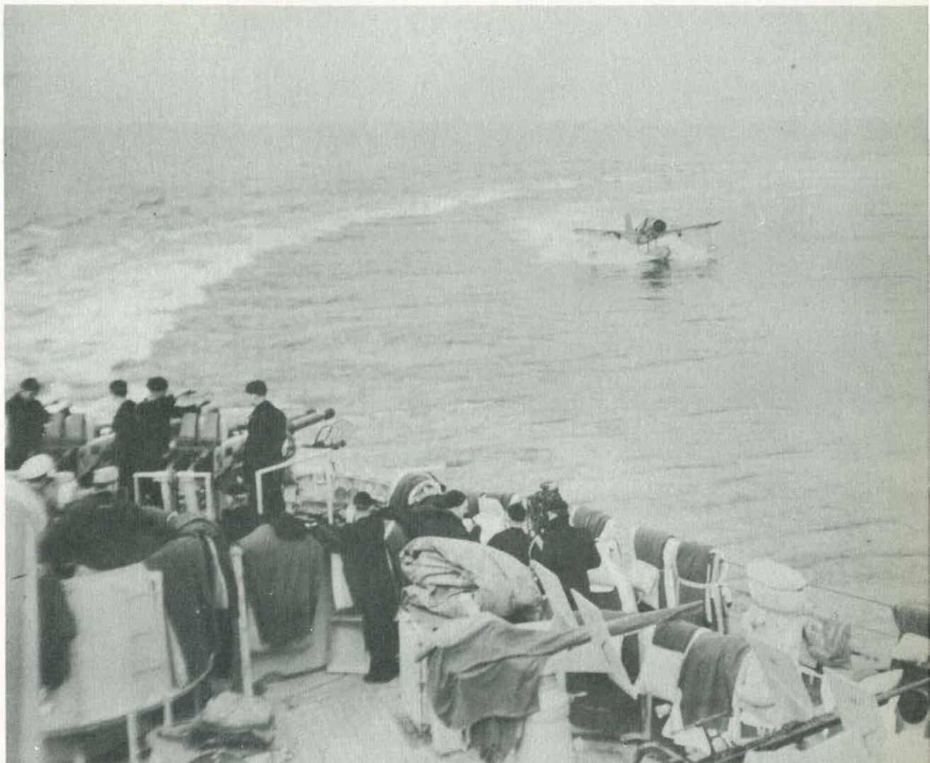
Ship swings hard to port to create slick for a "Charlie" recovery of an OS2U.
