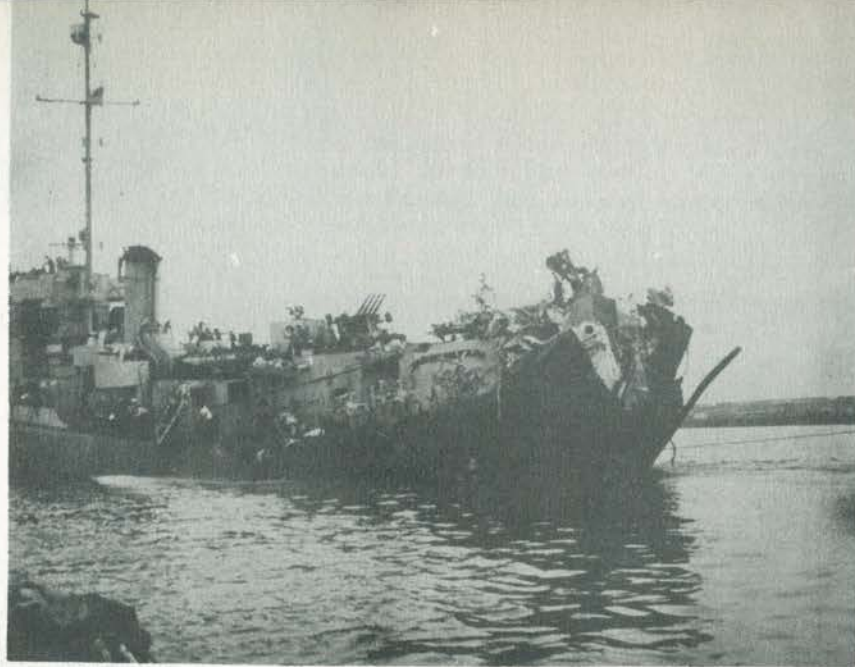
Torpedo Damaged USS Barr Lies In Casablanca Harbor—Her stern a shambles of twisted wreckage, the destroyer escort USS Barr lies in the harbor at Casablanca, French Morocco, where she underwent temporary repairs to enable her to make the voyage back across the Atlantic to Boston. In an Atlantic action May 29, 1944 she was torpedoed by a Nazi U-boat. The escort carrier USS Block Island was sunk in the same battle. The Barr has now been converted into a transport.
