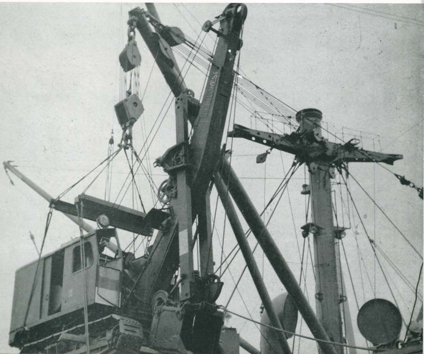
The "Jumbo" boom with a nice little draft of some sixty tons. It will land on the dock as gently as a sunbeam; an eager Seabee will promptly drive it away and start digging.
