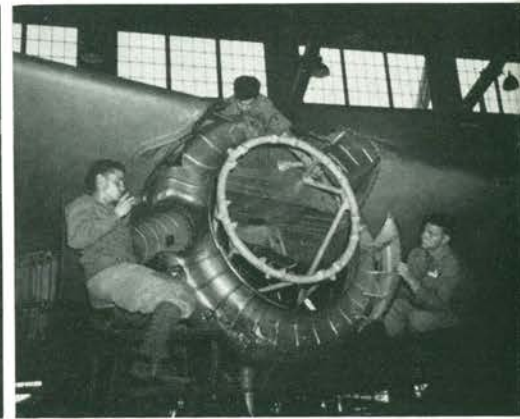
Removing Engine Mount Exhaust Shroud.
