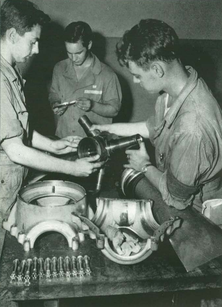
Disassembly of a Hydromatic Propeller.
