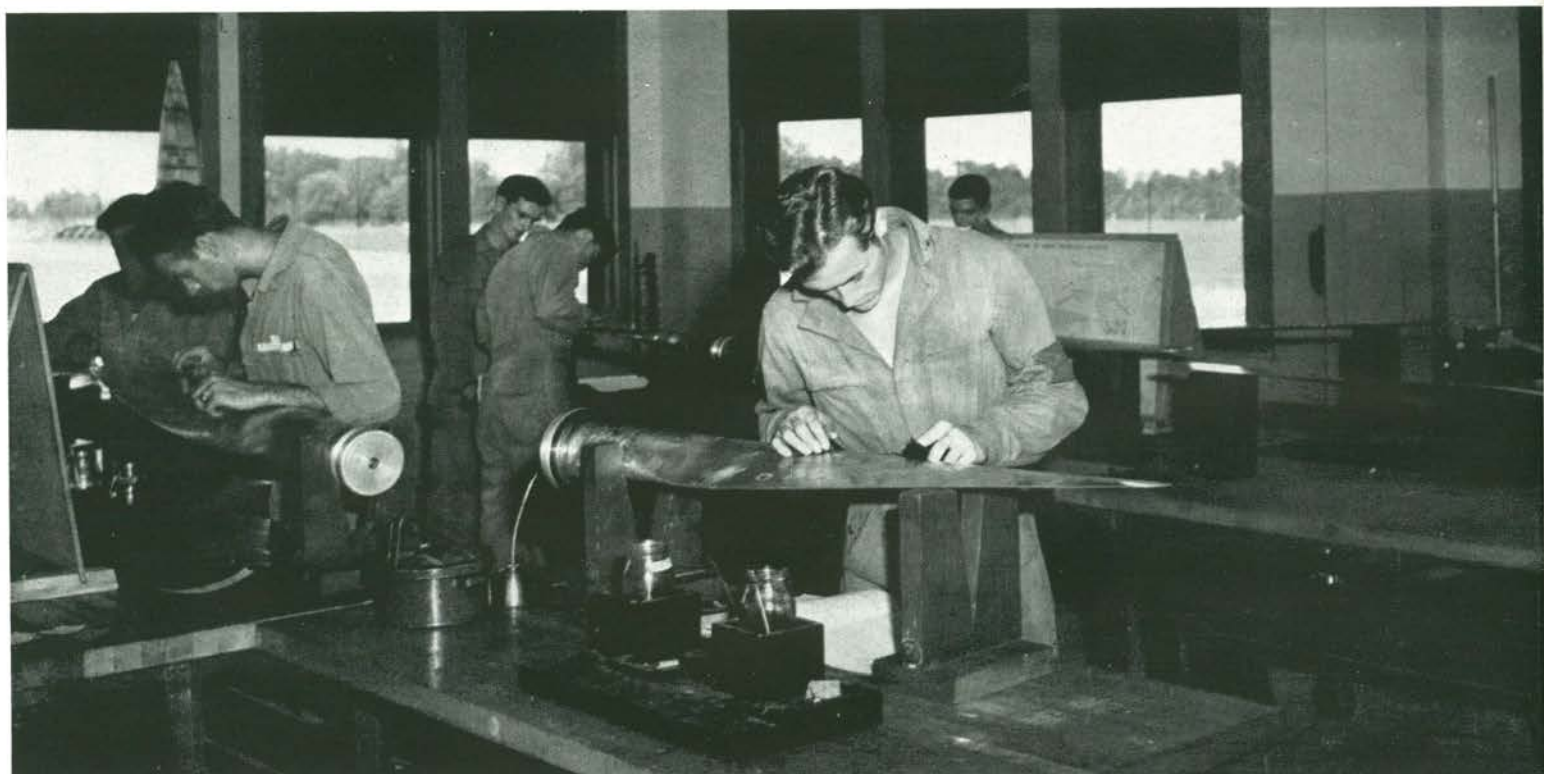
PROPELLER INSPECTION AND REPAIR
