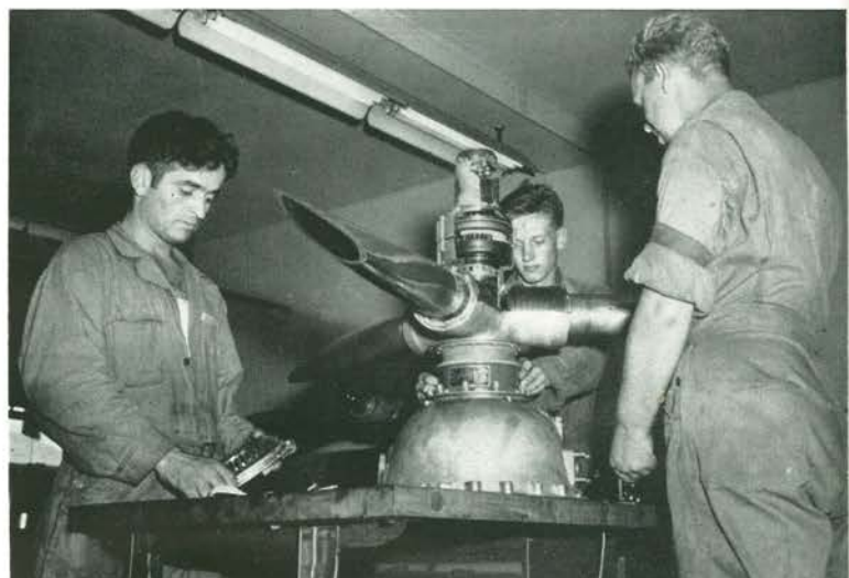
Cut-away Mockup of Curtiss Electric Propeller.
