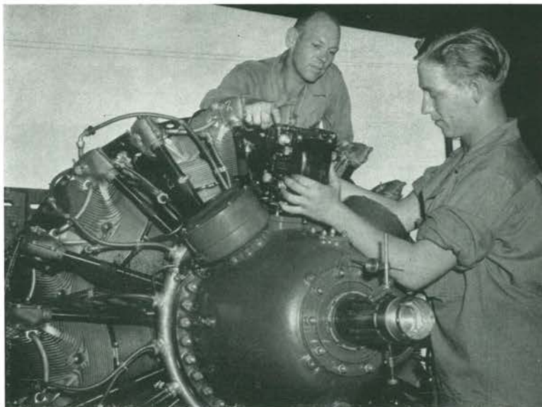
Ignition Timing on an R-2800 Engine.
