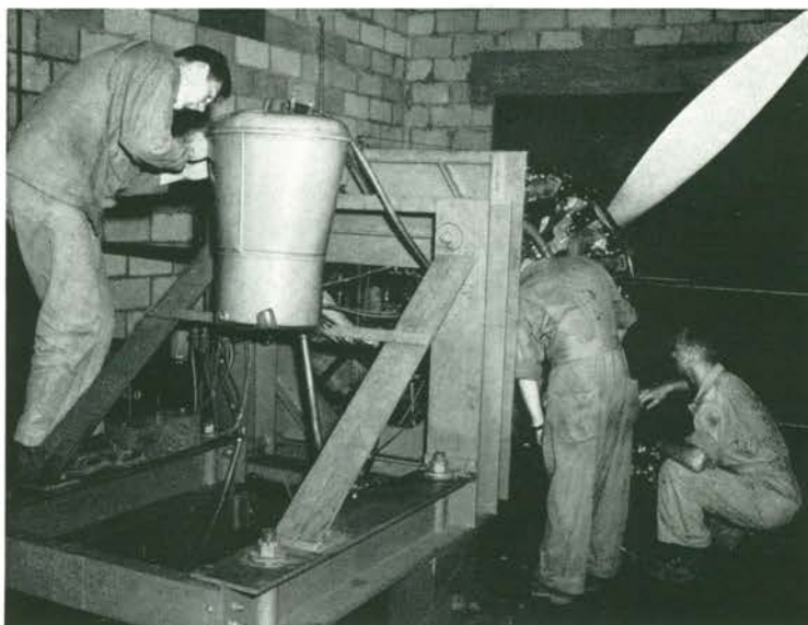
Pre-flight Inspection on R-2600 Engine.
