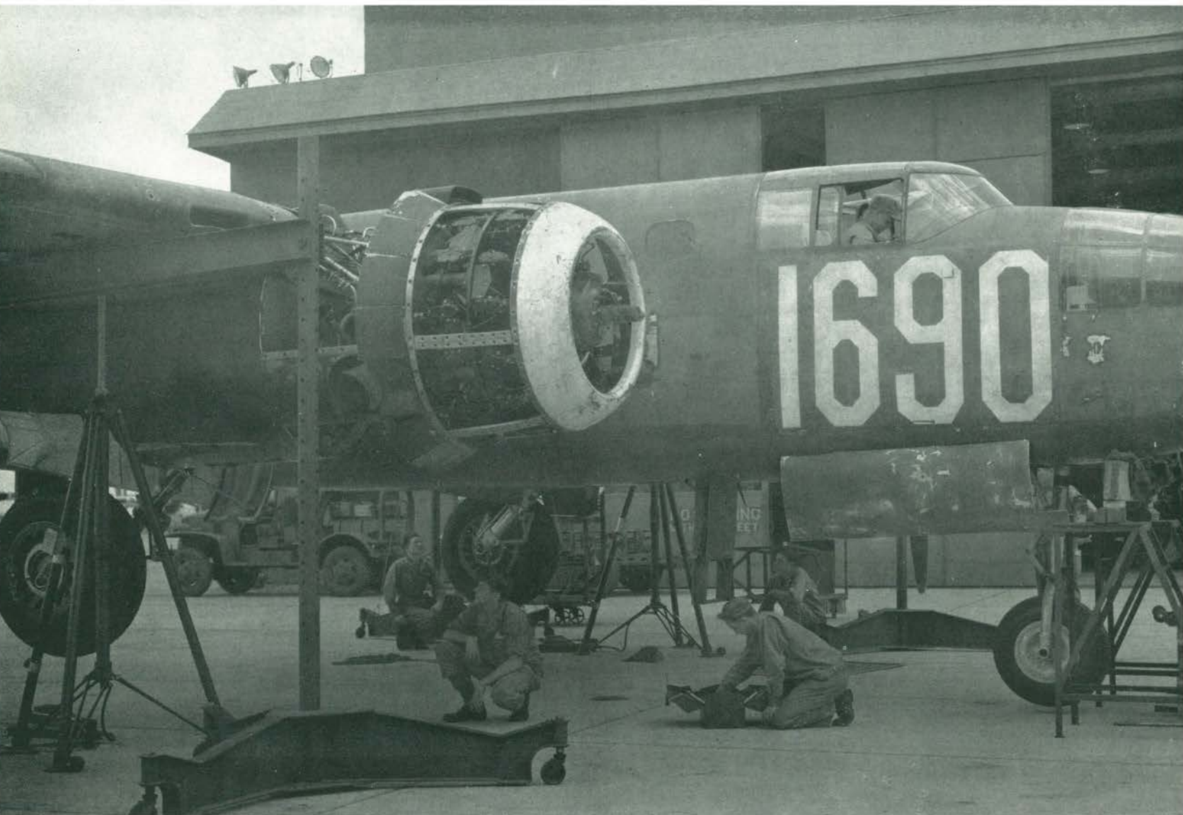
RETRACTION CHECK ON A B-25 PLANE
