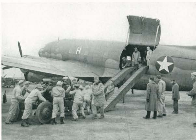
Experimental loading of 40 mm gun aboard C-47.
