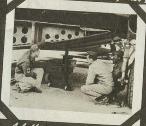
A bulky wing section is attached to lower fuselage of C-47 for rush shipment
