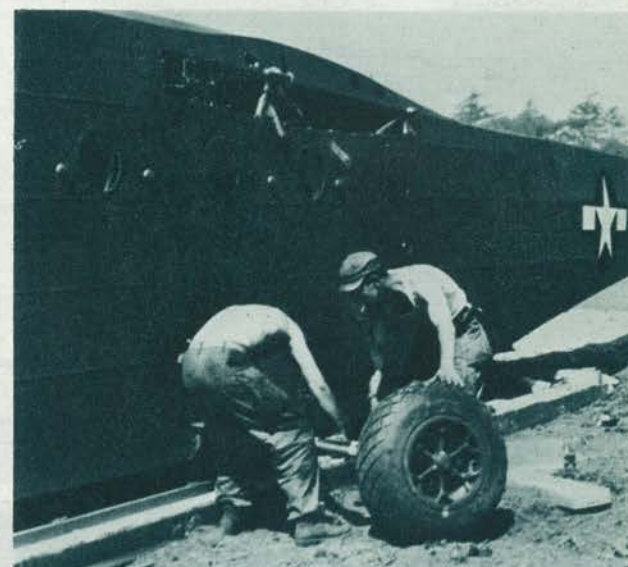
Fuselage completed, mechanics install the rear wheel of ship.
