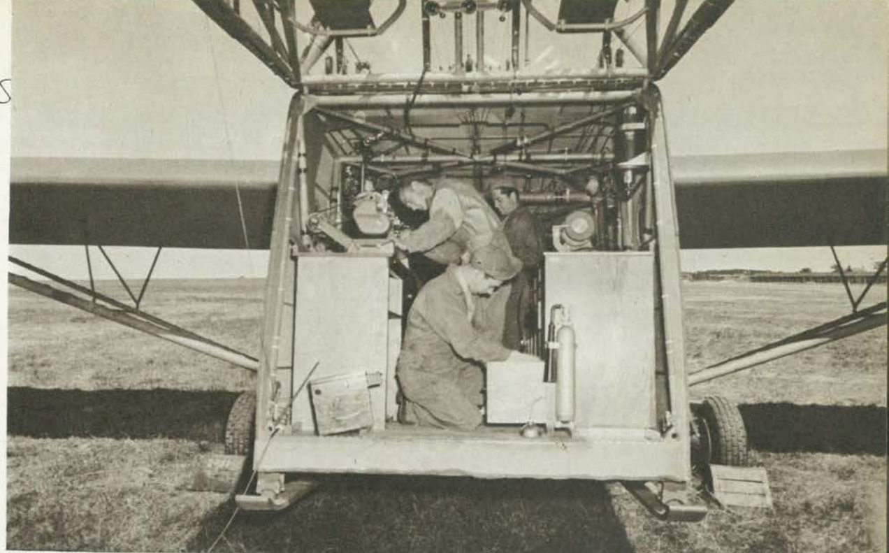
The "operations" cabin is a complicated looking affair. Mechanics making adjustments prior to attaching fuselage.
