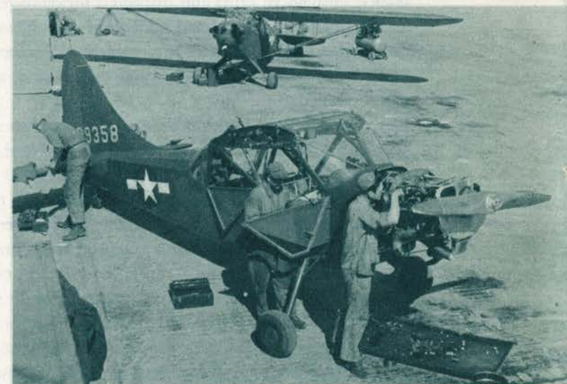
Aviation mechanics at work assembling a Piper Cub. After assembly, planes are inspected, tagged, made ready, lined up for test flight.
