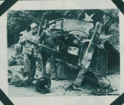
Salvaging usable parts of a badly damaged truck
