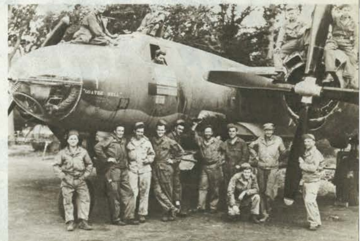
IX AFSC mechanics grouped around "Goatee Hell," a B-26 built wholly from two bombers badly wrecked in collision.
