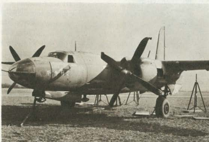
With jacks and balloons removed from under-wing, "Patches" is on her own feet, stands ready to be towed to the repair hangar.
