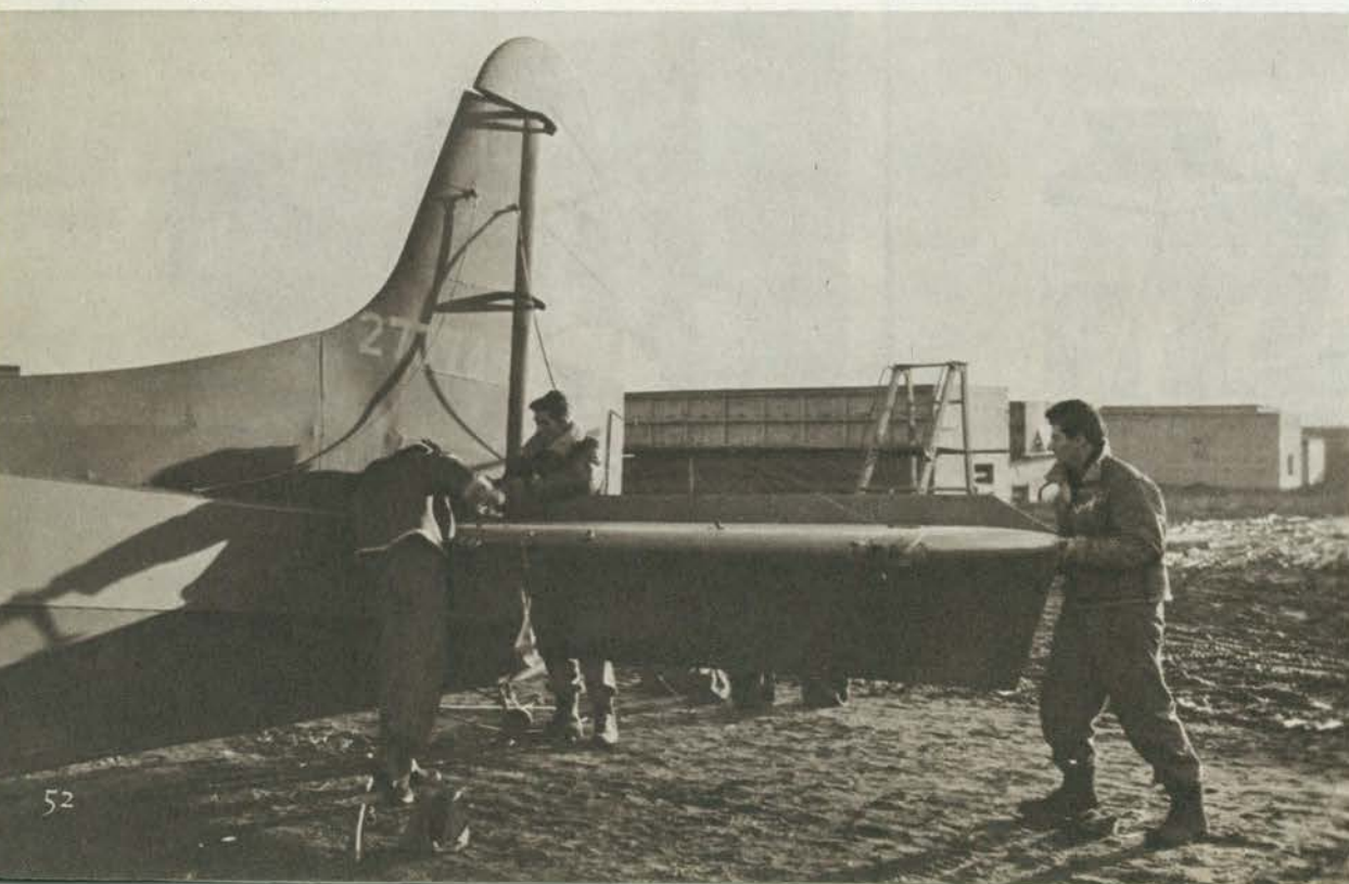
Empennage is placed into position after tail adjustments have been made. Wood is basic material used for gliders.
