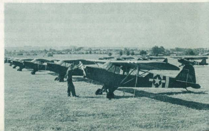
Aviation mechanics at work assembling a Piper Cub. After assembly, planes are inspected, tagged, made ready, lined up for test flight.
