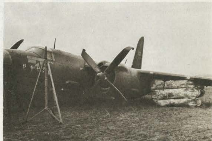
Deflated balloons are placed under each wing to raise 18 tons of combat aircraft to its normal height and lower the landing gear.
