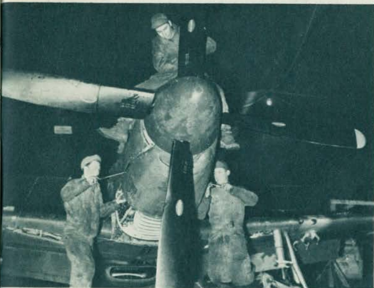
The cowling is installed on a Mustang approaching completion.
