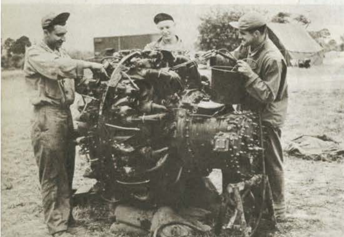
Before its return to the factory for overhaul , mechanics clean, overlay a P-47 engine with a film of preservative.
