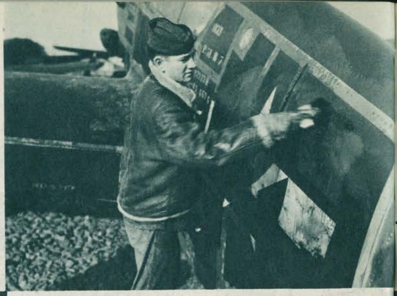
Removing the protective cosmolene coating from a P-51 Mustang.
