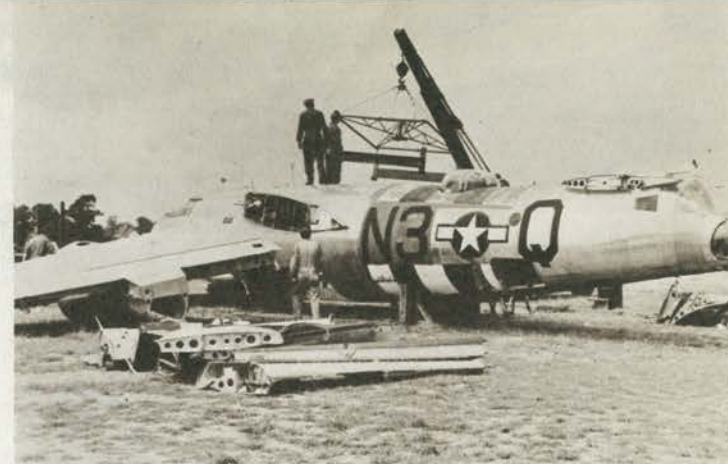
Wing and tail surfaces removed , this B-26 is ready to be put on trailer for removal to an air depot for either salvage or repair.
