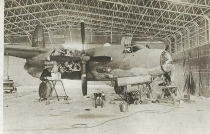
"Mary" Ninth Air Force B-26 Marauder, shown getting complete overhaul by mechanics of IX AFSC. Work went on 24 hours daily.
