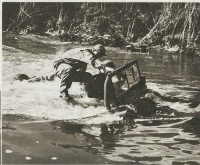
This is not an amphibious craft—just a jeep which has been thoroughly waterproofed!
