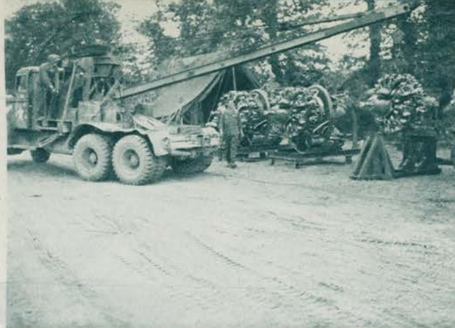
Thunderbolt engines are being placed in crates prior to overhaul.
