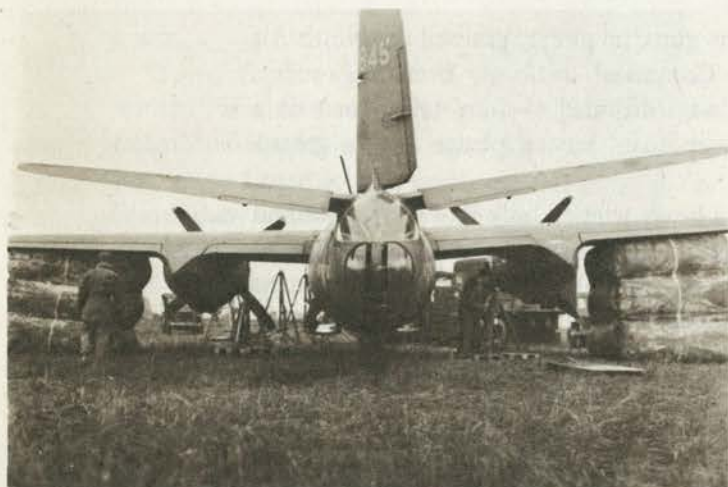
Balloons are inflated and the crew are seen placing jacks in position. Jacks relieve some of the weight imposed on the balloons.
