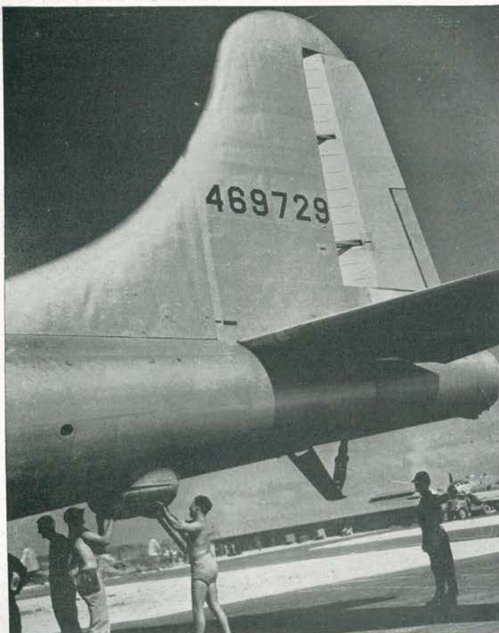
TAIL. Two crewmen slip the tail-belly turret into place as the ground crew buttons up the great ship for the next Jap strike, which will get under way as soon as flight crew arrives from briefing room. These missions were taken quite seriously by crews.
