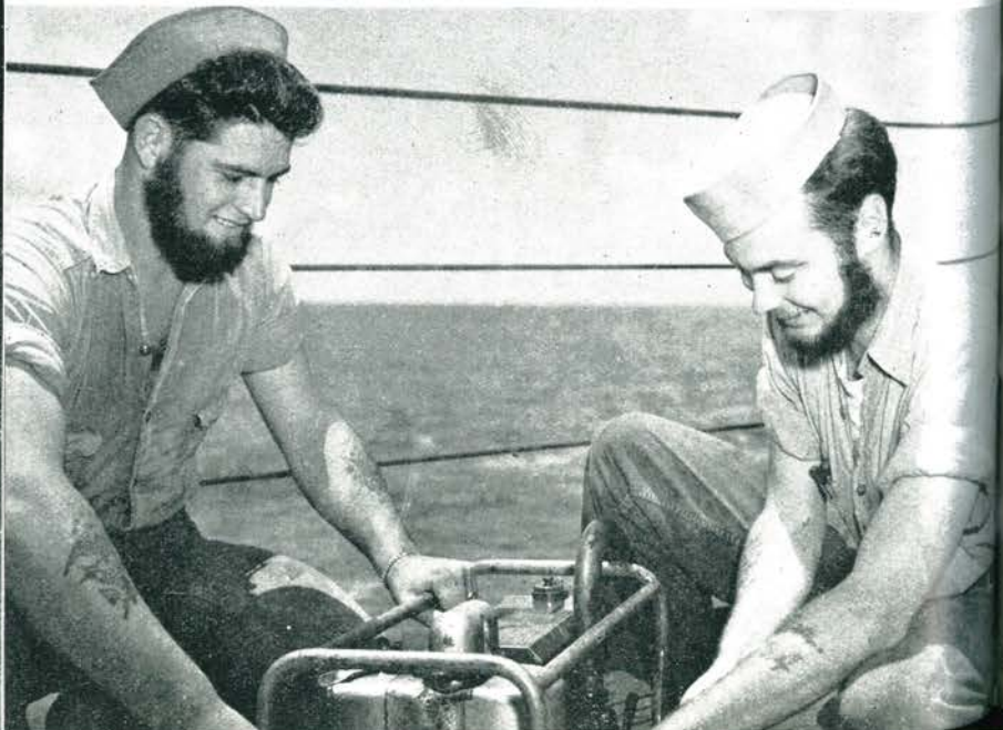
REPAIRING A "HANDY BILLY"
