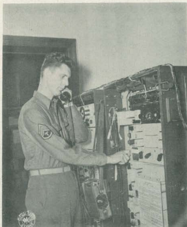
Above: Chester Smith checking a C-F-1A Carrier, a power booster on long lines. At right: Dambrogio, Bockmeyer and Hanson fiddling with antenna array at a radio installation.
